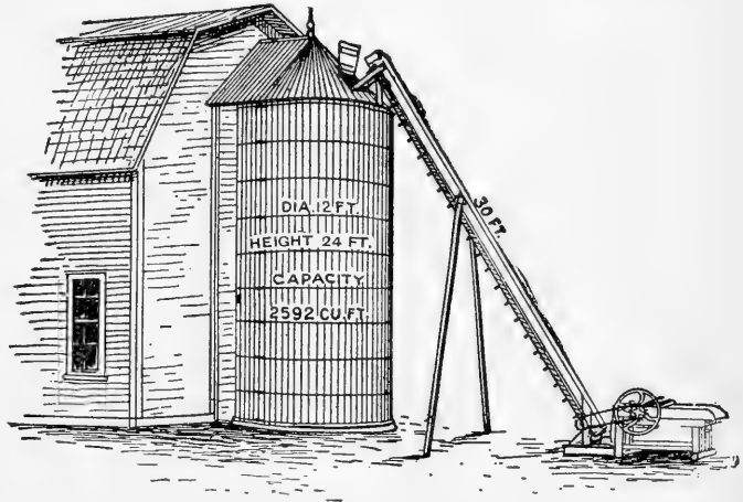
FIG. 169. Stave silo, 12 feet diameter, 24 feet high; capacity, 50 tons. (Elias.)
